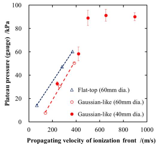
Fig.6 Relationships between propagating velocity and wall pressure at the focusing reflector.
