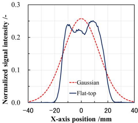
Fig.3 Beam profiles. (Gaussian: calculation, Flat-top: measurement by low-power test system)
