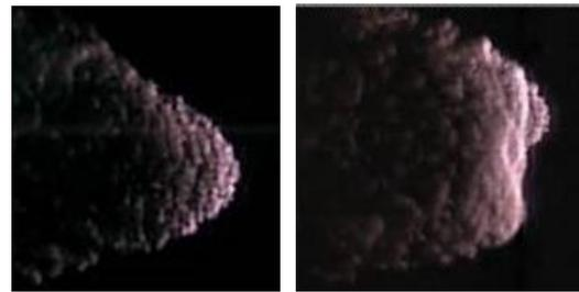
Fig.5 Short exposure images taken by a fast-framing camera (exposure time: 1000 ns, left: Gaussian-like, right: flat-top, beam direction: from right to left)
